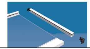
**6.** Once you have assembled the flyscreen frame you can now raise it into place. This is a two person job. Position and then screw into the frame work of your doorway with the four screws provided. Now attach the plastic covers over screw holes.
