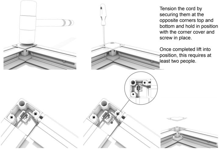
Screw the corners into the door frame. Only then release the tape and pull the screen to the shut position.
