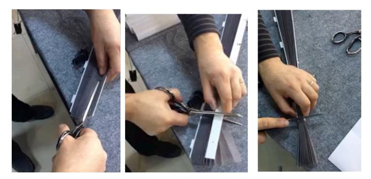
Cut the white plastic backing on the mesh screen with scissors by 0.5cm on both sides so that it will sit in the corners correctly.
