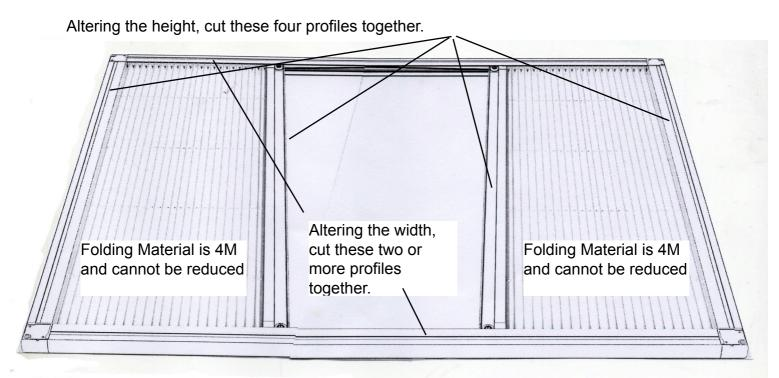
Altering the height, cut these three profiles together. Then construct the frame without the screen to ensure it fits around the doorway.
