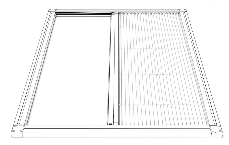
To alter the width of the screen cut the top and bottom profiles to the required width. Always allow for the corners which measure 4cm each.
