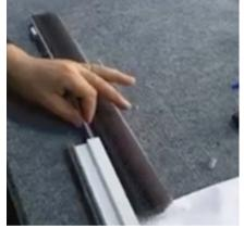
Cut the metal profiles 4cm less than the required height to allow for the corners. Cut the mesh screen 3cm less than the required height.
