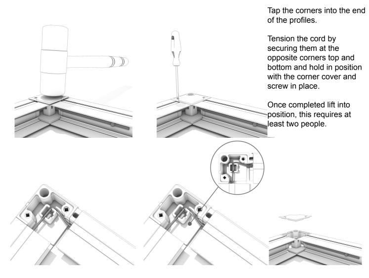
Screw the corners into the door frame. Make sure it is square. Only then release the tape and pull the screen to the shut position. You should check and retension the cords
