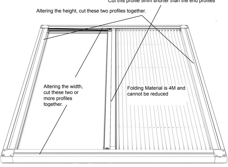
Altering the height, cut these two end profiles together. Then the middle screen profile 5mm less than the two end profiles. Then construct the frame without the screen to ensure it fits around the doorway. do not release the screen material, keep it secured until fixed in position.
